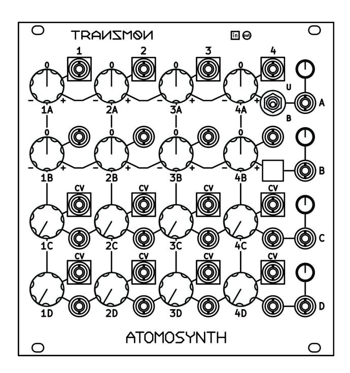
The Atomosynth Transmon is a 4-input and 4-output matrix mixer eurorack module, featuring 8 bipolar attenuators and 8 individual VCAs, and many other utilities, it gives you great flexibility for mixing, controlling, and routing Audio or Voltage with a small footprint.
